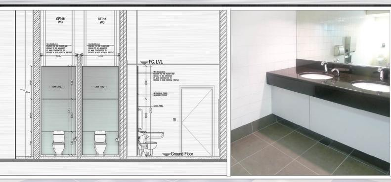
HIGHLY DURABLE, WATER AND IMPACT RESISTANT, DUR TOILET FLUSH TANK CLADDING, VANITY COUNTERS AND FASCIA PANELS ARE MADE OF HPL, MOUNTED ON ALUMINUM PROFILES. THE SYSTEM IS RIGID AND FLEXIBLE TO REMOVE FOR MAINTENANCE, MAKING IT A PERFECT SOLUTION FOR HIGH END INSTALLATIONS.
